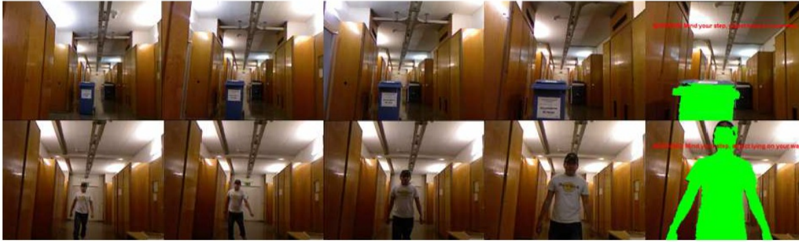
Figure 2. While a blind individual explores an environment (probably with the global module), the alerting system senses if any object approaches dangerously (e.g. a crash can, or a person). Note that the alerting system says nothing about the nature of the object; it just triggers an alarm indiscriminately.
