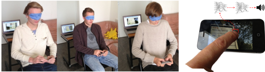
Figure 4. Blindfolded individuals detecting bus numbers with the text recognition engine. At the rightmost, we can see closely the way it works: a first neural network classify whether the finger is touching on text. If so, a second network classifies the particular letter being touched.
