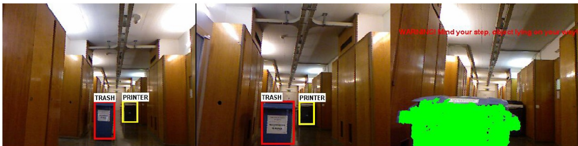
Figure 3. The recognition module informs about the presence of previously learned objects by voice, e.g. Trash! Printer!. Note that in the rightmost frame, one of the objects became dangerously close hence, detectable by the alerting system.
