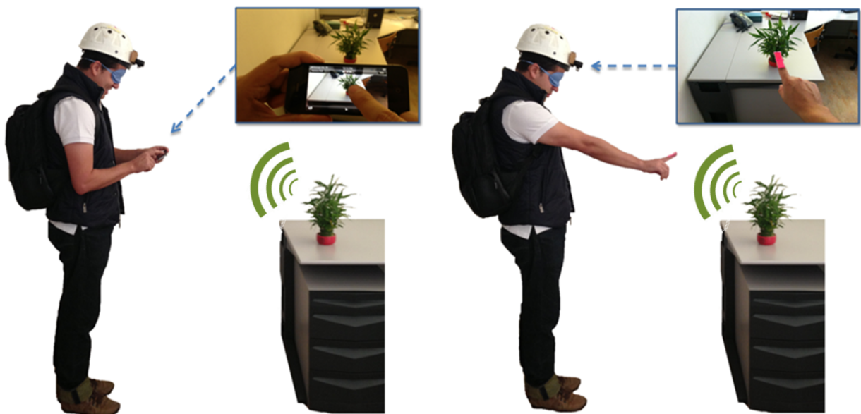
Figure 1. Blindfolded individual exploring a scene using the global module with (left) and without (right) a tactile tablet. In both cases, the sound being activated is that of green (plant leaves). Also, the sound is heard as though coming from the actual plant location in space (virtual source). Note that without a tablet, the object (e.g. plant) will also emit sound if touched (tactile sensation augmented by hearing).
