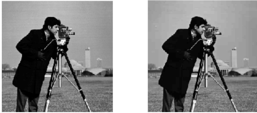
Figure 1: Example for image compression. Left: original image. Right: Compressed image only requiring around 5% of the storage required for original image.
